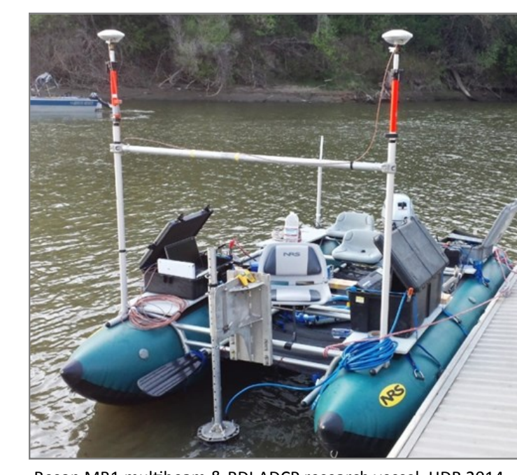
Reson M81 multibeam & RDI ADCP research vessel, HDR 2014
