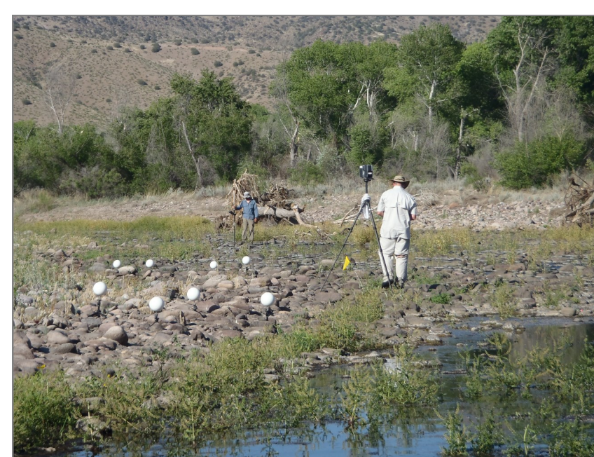
RTK survey and Faro laser scanning, New Mexico. HDR 2014
