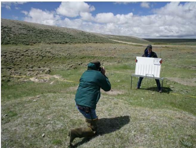
We collected data from an erosion bridge (also called a pin meter), by photographing pin height as shown above. We used ImageMeasurement to measure pin height above the leveled bar from the photographs. We calculated the pin-height standard deviation which we used as a surface roughness index (SRI).
