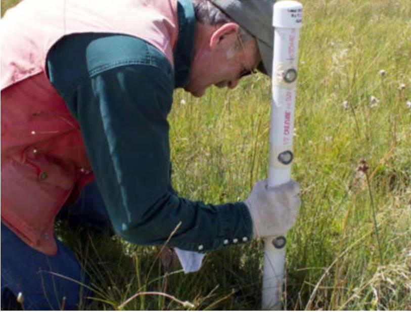
The sensors were enclosed in PVC housings as shown above, and the housings inserted into the soil profile to the desired depth as shown below.
